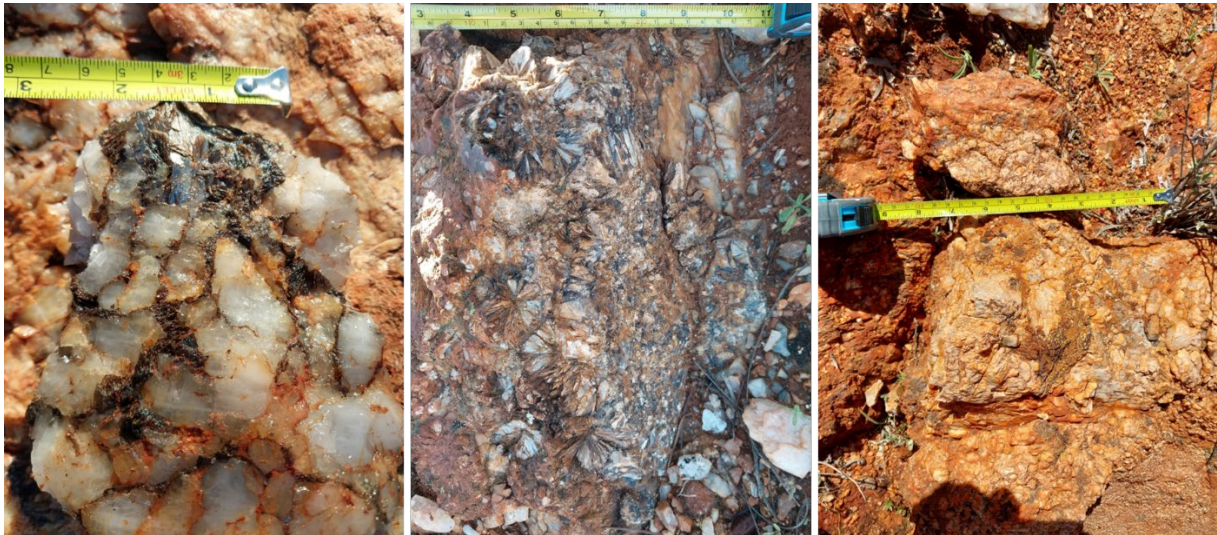
LEFT: QUARTZ, FELDSPAR, MUSCOVITE PEGMATITE (0.40% Li 2 O, 364PPM Cs, 46PPM TA). MIDDLE: QUARTZ, FELDSPAR, MUSCOVITE PEGMATITE (0.33% Li 2 O, 265PPM Cs, 13PPM TA). RIGHT: QUARTZ, FELDSPAR, MINOR MUSCOVITE PEGMATITE (134PPM Cs, 257PPM TA, 856PPM BE)
