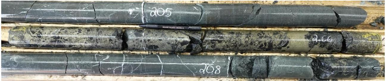
Figure 3: Brecciated Semi-massive VMS intercept 206.24-206.95m
