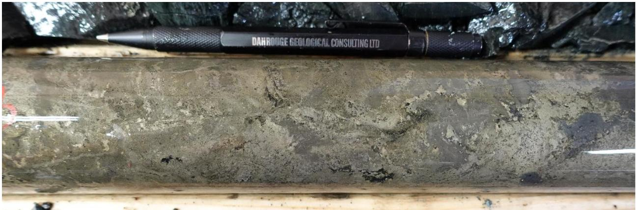
Figure 2: YH24-123 153.2m to 153.4m Sulphide intercept
