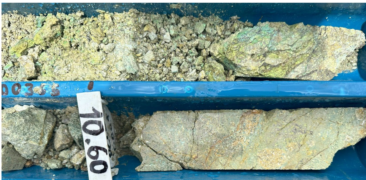
Figure 4: Example of secondary copper mineralisation at around 9.70m depth at Cumbre Coya Target 23PCCD0001
