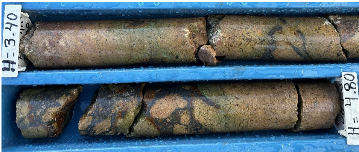
Figure 3: Example of secondary copper mineralisation at around 4.5m depth in 23PCMD0001
