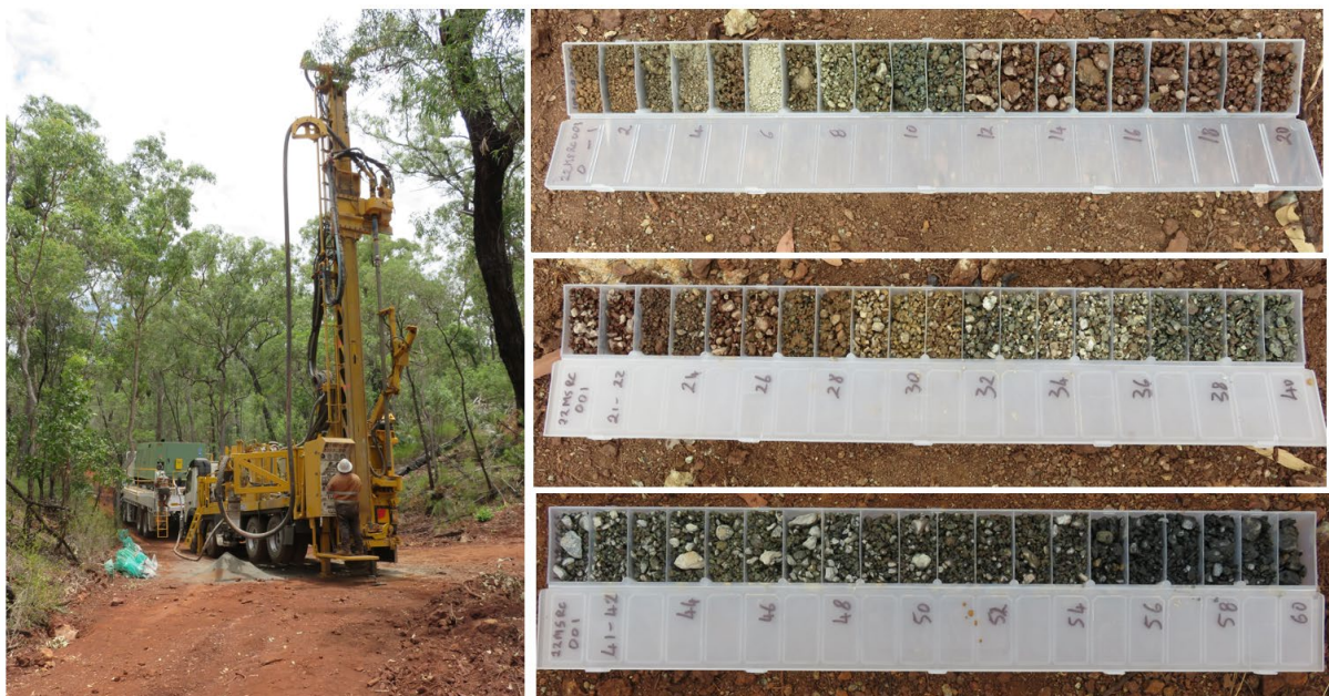
FIGURE 2: DRILL RIG OPERATING AT MT SLOPEAWAY IN LATE 2022 (LEFT HAND SIDE); REPRESENTATIVE CHIP TRAY SAMPLES ILLUSTRATING LATERITIC HOST ROCK PROFILE IN 22MSRC001 (RIGHT HAND SIDE)
