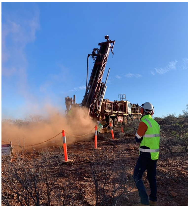
FIGURE 4: RC RIG DRILLING FIRST COLLAR AT JOHNSON WELL.
