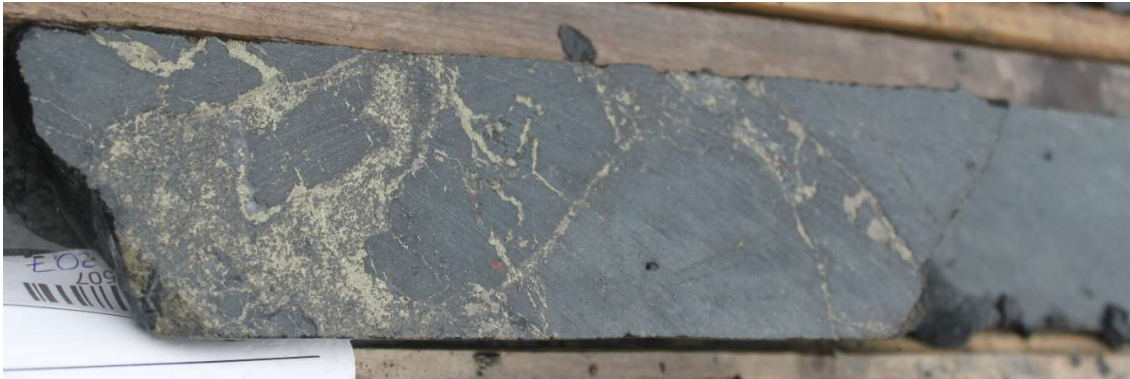
Figure 2: YH22-078 cut section of previously unsampled core, showing Chalcopyrite, Pyrrhotite and Pyrite (Inset of above)
