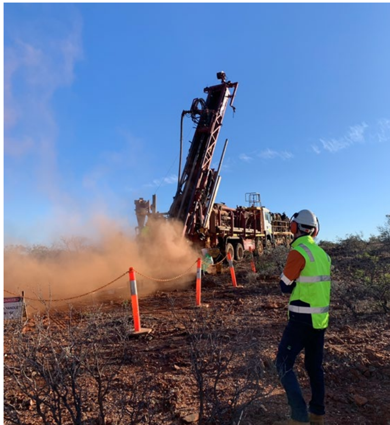
FIGURE 6: RC RIG DRILLING FIRST COLLAR AT JOHNSON WELL
