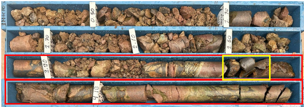
FIGURE 3: PICHA PROJECT – HIGH-GRADE COPPER-SILVER MINERALISATION AT COBREMANI TARGET (24PCMD0003 – 5.12M @ 5.4% CU AND 44.9G/T AG FROM 2.88M)
