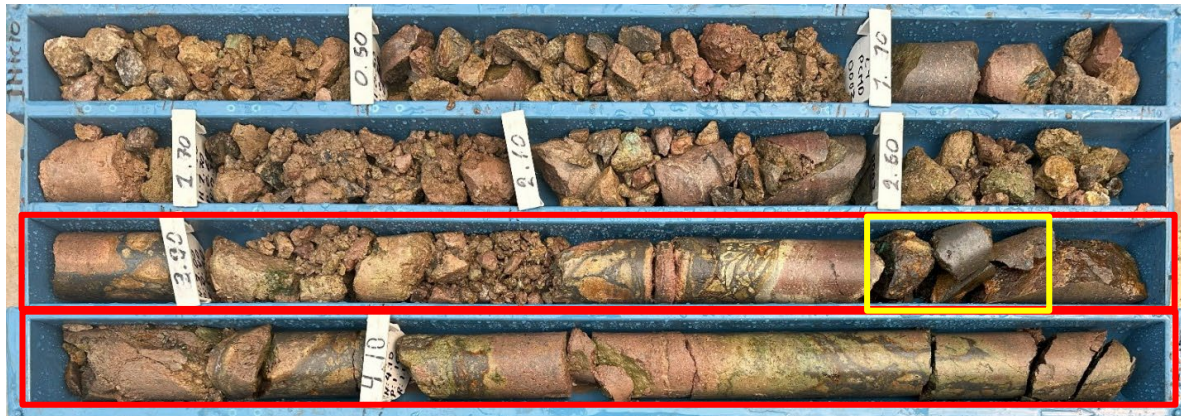
Figure 6: Picha Copper-Silver Project – high-grade copper-silver mineralisation at Cobremani target (24PCMD0003 – 5.12m @ 5.4% Cu and 44.9g/t Ag from 2.88m)
