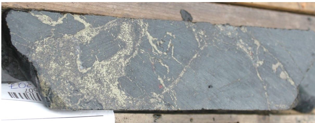
Figure 1: YH22-078 cut section of previously unsampled core, showing Chalcopyrite, Pyrrhotite and Pyrite 2
